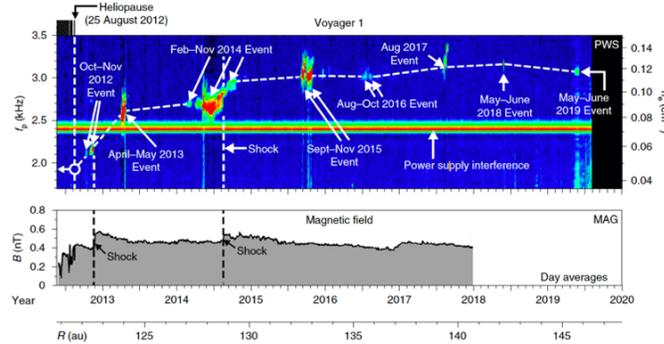
Figure 1: Frequency-time spectrogram of electron plasma oscillations detected by the V1, and the corresponding local magnetic field strength from the magnetometer. Two vertical dashed lines indicate two observed shocks in the VLISM. (from Gurnett & Kurth 2019).
