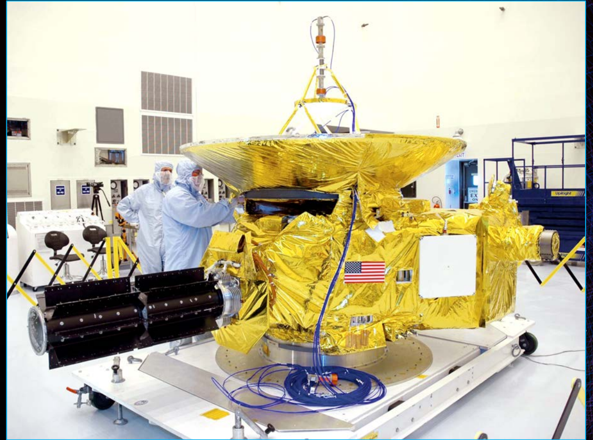
New Horizons with GPHS-RTG – Now in 14 th year Voyager MHW-RTGs now in 43 rd year
