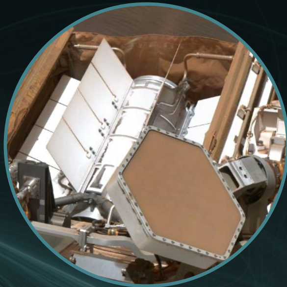
MMRTG Multi-Mission Radioisotope Power System
